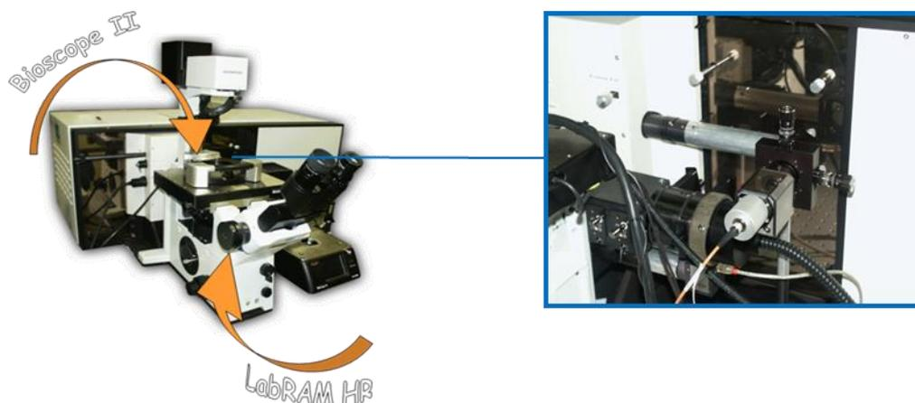
**Fig. 1** AFM/DFS/Raman instrument with a magnification of the accessory for TIR light injection.
